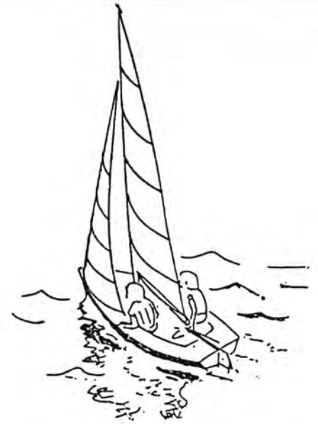
Figure 6: Fastest trim, 3 knots wind, wave 1-2 foot. Sails everywhere about 15% camber, for maximum possible power, sheeted as wide as necessary, virtually no twist.
