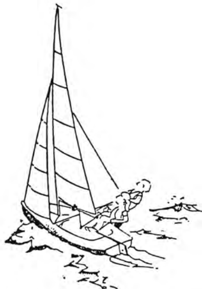
Figure 2: Preferable strong-wind trim; main flattened for minimum drag in lulls, jib eased until mainsail backwind just appears in the strongest pulls
