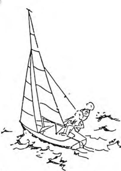
Figure 1: Laser II sailing on a jib and leech of main with jib sheeted firmly and mainsail eased to keep boat upright. This commonly-accepted trim for "survival" winds is slow.
